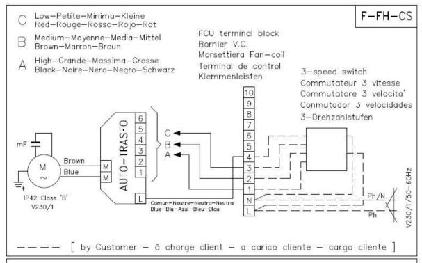
DO NOT CONNECT IN PARALLEL DIFFERENT MOTORS —NE PAS CONNAITRE EN PARALLELE MOTEURS DIFFERENTS
